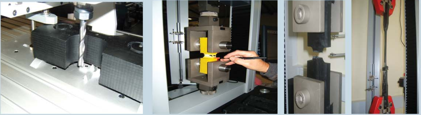
The above photographs show samples cut with the Model 2 CNC, under actual test conditions
