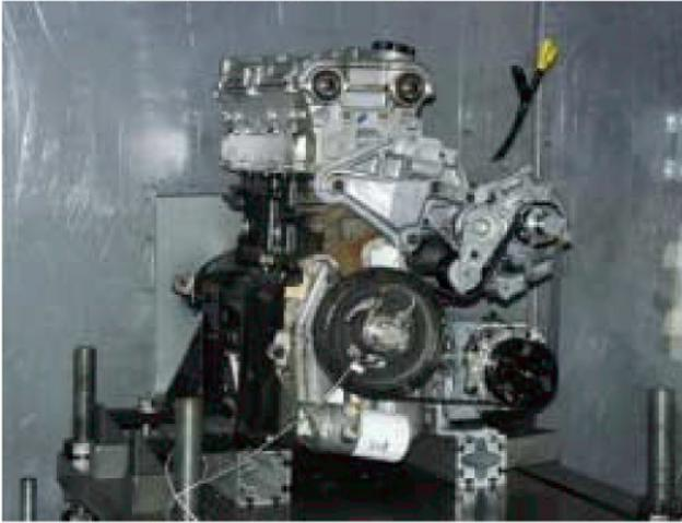
**Team Engine Simulation System set up for testing a Front Engine Accessory Drive system. The ESS is behind the wall in the background to facilitate noise mapping of the FEAD during testing.**
