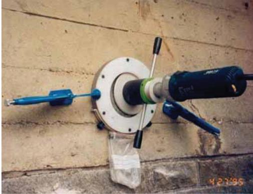
The **Profile Grinder** is ready for grinding on a 1-year old wall. The powder obtained for each depth increment is collected in a separate plastic bag. Chloride content at each depth is determined on-site using the **RCT**.
