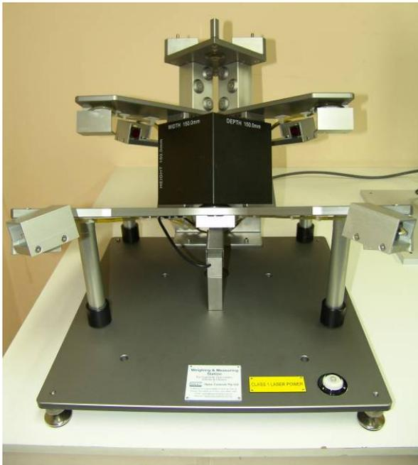
**Spacer Jig locates on the top plate of the station**
